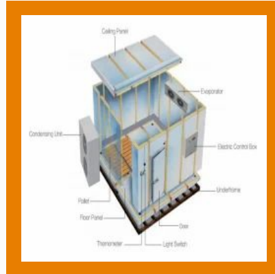
Cold Room Structure
